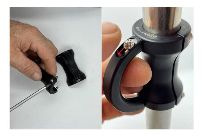
NB: tighten the screws slightly one after the other, then lock one by one gradually. Tighten with the short part of the ALLEN wrench so as not to break the screws.
