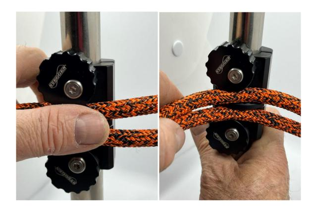
TIP: adjust the angular orientation of your rope blocker with the face of the jaws in line with the bow: the engagement of the rope will be all the more fluid!
