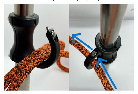
TIP: It is possible to use the body of the fairlead as a friction ring if the line angle is too open: on multihulls, to guide the line from the bowsprit via the starboard or port hull, this trick is essential!
