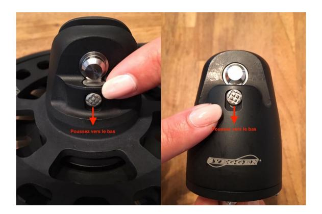
After rinsing, you can oil this mechanism at the end of the season, winch ratchet oil, armory or other, it is possible to unscrew the knurled knob and remove the bushel for maintenance: to be reassembled with TEFGEL or marine grease.
